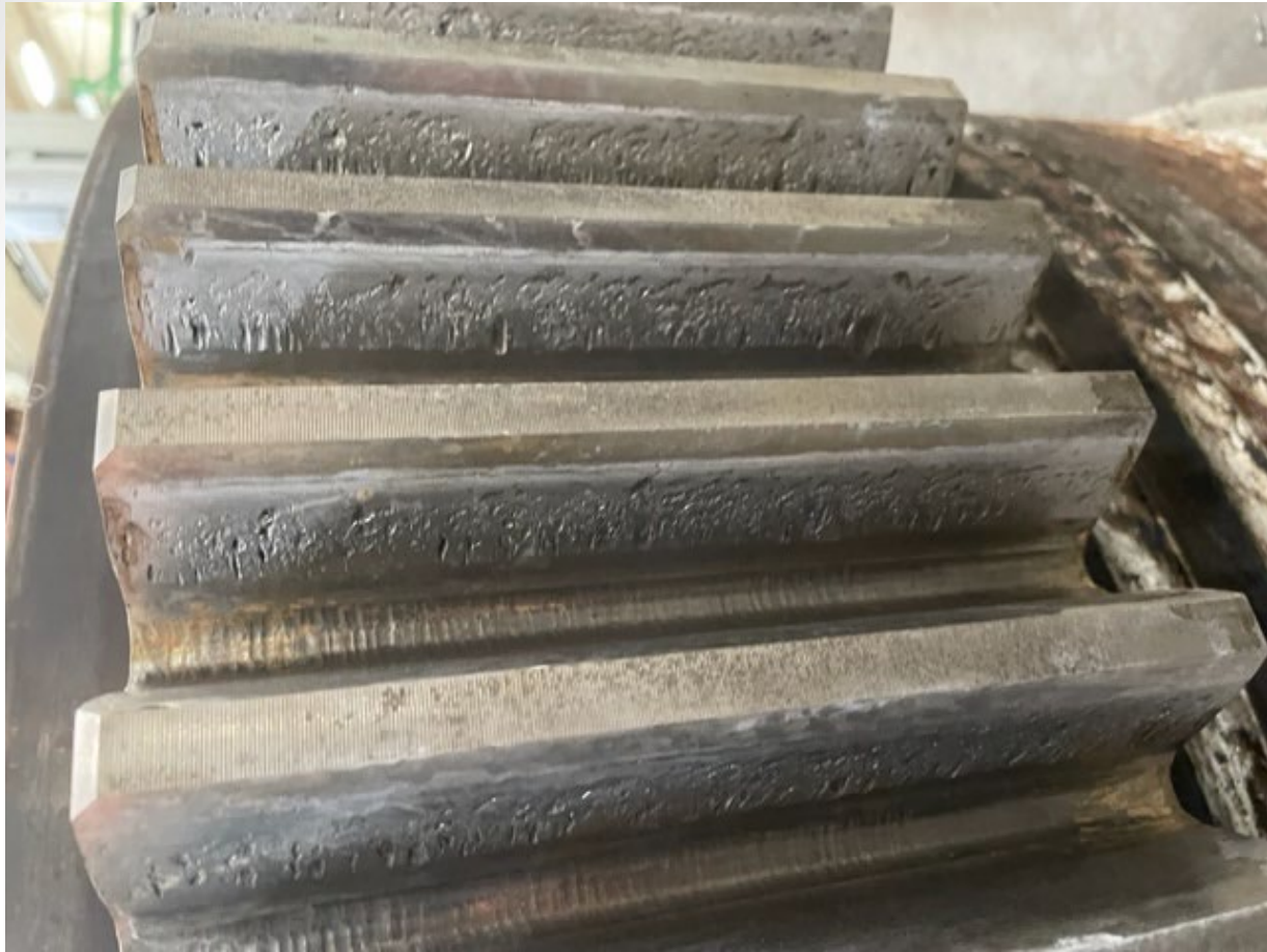
Pitted north drum gear
